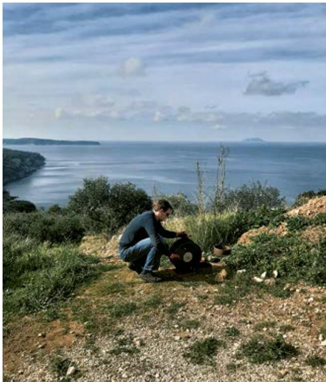
Mjerenje razine podzemne vode u bušotini V-1 iznad Velog žala (foto M. Bašić)
