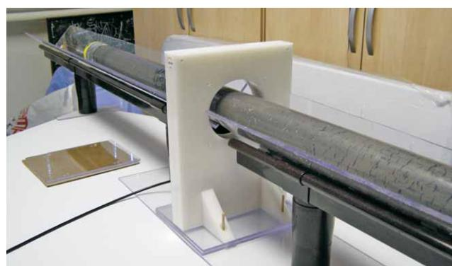
Mjerenje magnetske susceptibilnosti na jezgrama pomoću MS2 (Bartington Instruments) s MS2C senzorom. • Measurement of magnetic susceptibility in cores using Bartington Instruments MS2 with MS2C sensor.
