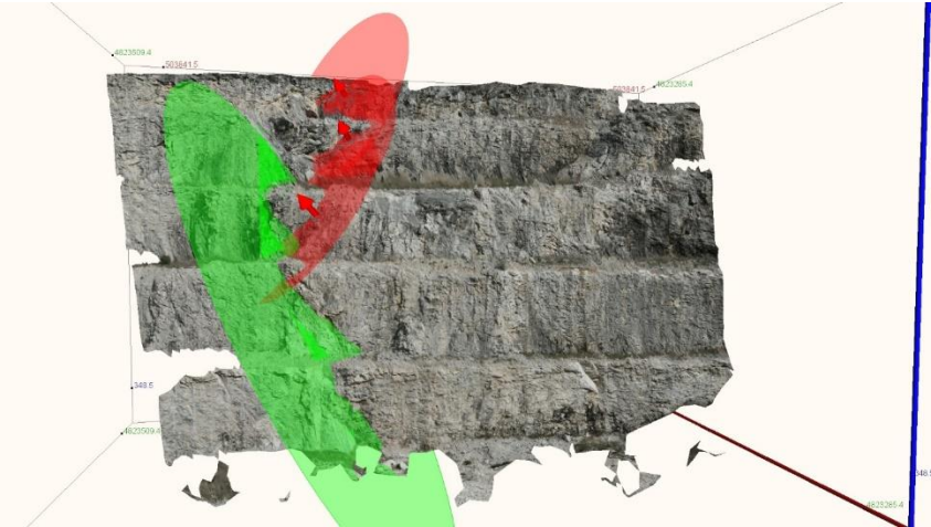
Slope on the eastern side of the quarry "Klis-Kosa" in the Upper Jurassic - Lower Cretaceous limestones with indicated faults related to block instabilities - wedges.
